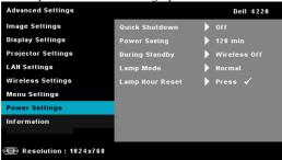
QUICK SHUTDOWN—Select On to turn off the projector with a single press of the Power button. This function allows the projector to quickly power off with an accelerated fan speed. Slightly higher acoustic noise is expected during quick power off.
