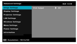
**VGA OUTPUT**—Select On or Off the VGA output function at projector standby status. Default is Off.
