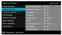
**FREQUENCY**—Allows you to change the display data clock frequency to match the frequency of your computer's graphics card. If you see a vertical flickering wave, use the Frequency control to minimize the bars. This is a coarse adjustment.
