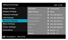
**NOTE:** If your want to use the wireless connection for 4220 or 4320 projector, need installed the optional wireless dongle. See "Installing the Optional Wireless Dongle" on page 11.
