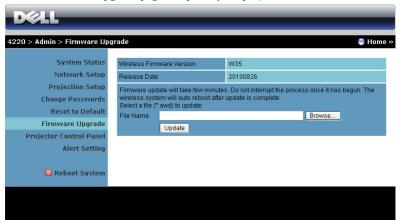
**NOTE:** Please disable and enable wireless/network using the OSD to restart the network card for the projector after firmware upgrade is successful.
