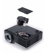
Setting menu on page 54). When a new lamp module has been changed, the projector will automatically detect and reset the lamp hours.
