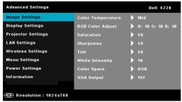
**COLOR TEMPERATURE**—Allows you to adjust the color temperature. The screen appears cooler at higher color temperatures and warmer at lower color temperatures. When you adjust the values in the Color Adjust menu, the Custom mode is activated. The values are saved in the Custom mode.
