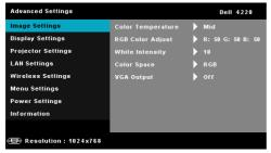
**COLOR TEMPERATURE**—Allows you to adjust the color temperature. The screen appears cooler at higher color temperatures and warmer at lower color temperatures. When you adjust the values in the **Color Adjust** menu, the Custom mode is activated. The values are saved in the Custom mode.
