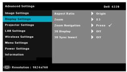
**ASPECT RATIO**—Allows you to select the aspect ratio to adjust how the image appears. Options are: Origin, 16:9, and 4:3.
