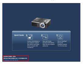
**NOTE:** If wireless connection is disabled, then follow these steps to set up: ADVANCED SETTINGS → Wireless settings → Wireless → Connected. The image input source will be automatically switched to wireless screen when wireless option is selected in this step.
