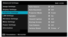
**AUTO SOURCE**—Select Off (the default) to lock the current input signal. If you press the Source button when the Auto Source mode is set to Off, you can manually select the input signal. Select **On** to auto detect the available input signals. If you press the Source button when the projector is on, it automatically finds the next available input signal.
