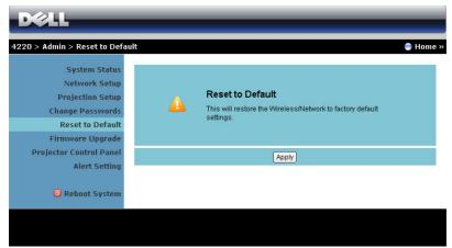
Click the **Apply** button to restore the wireless/network setup to its factory default settings.
