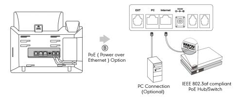
**Note** If in-line power switch/hub is provided, you don't need to connect the phone to the power adapter. Make sure the switch/hub is PoE-compliant.
