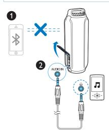
1 Open the protective cover on the bottom of the speaker.
