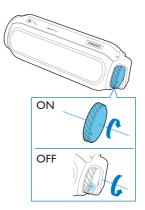
To turn the speaker on or off, rotate the knob clockwise or anticlockwise until you hear a click.
