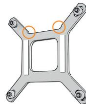
**Ensure with LGA 1150/ 1151/ 1155/ 1156 sockets that when fitting the Intel® backplate it lies within the recesses on the backplate.**
