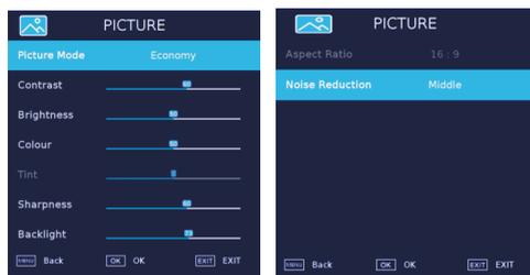
1. Press [▼] / [▲] to select: Picture Mode/Contrast/Brightness/Colour/Tint/Sharpness/Color Temperature/Aspect Ratio/Noise Reduction.
