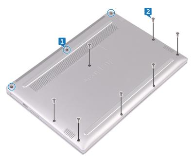
Using your fingertips, pry the base cover off the palm rest and keyboard assembly.
