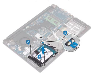
4 Disconnect the interposer from the hard-drive assembly.
