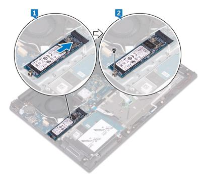
**NOTE:** Align the screw holes on the solid-state drive bracket to the screw holes on the solid-state drive, if applicable.
