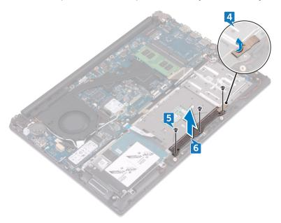
Remove the four screws (M2x2) that secure the touch pad to the palm rest and keyboard assembly.
