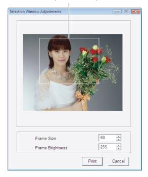
When you click the [Print] button, the portion of the image specified by the selection window is printed using the  $5 \times 5$  cell layout. Select the image with the best gray balance from the 25 images that are printed, and enter the X and Y coordinates (X,Y) printed under that image for the [X] and [Y] settings.
