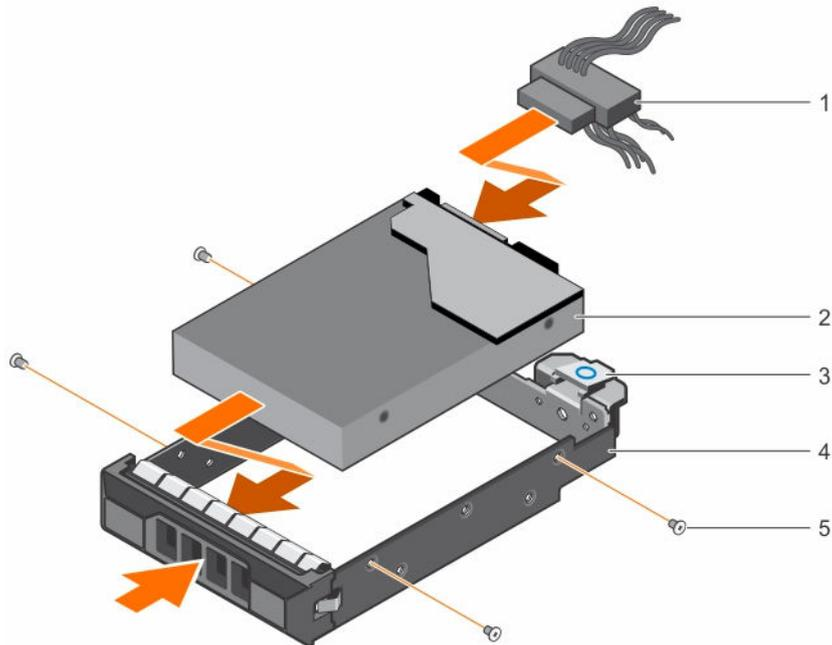
**Figure 33. Installing a cabled hard drive carrier**
