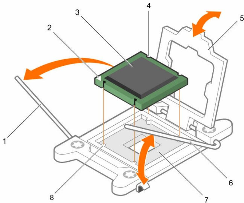
**Figure 66. Removing a processor**
