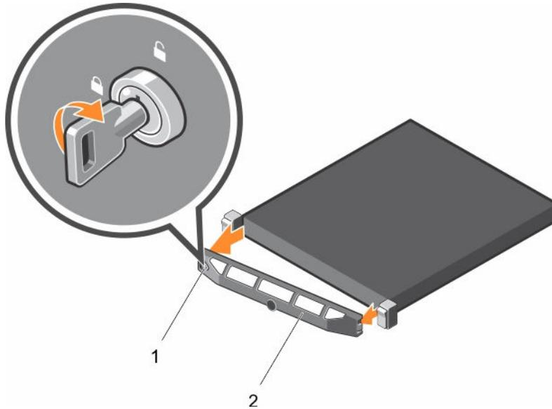
Figure 17. Removing the optional front bezel
