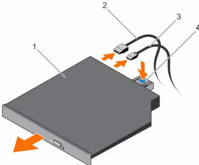
Figure 42. Removing the ultra slim optical drive
