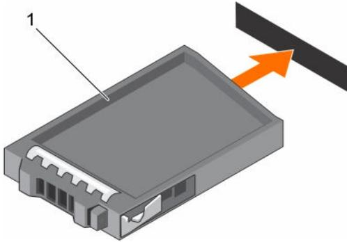
**Figure 29. Installing a 2.5-inch hard drive blank**
