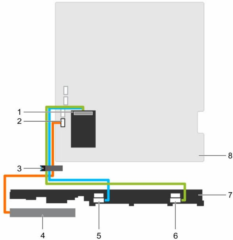
**Figure 81. Cabling diagram—Eight 2.5 inch SAS/SATA backplane**
