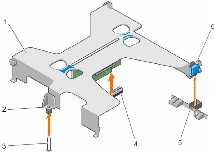
**Figure 50. Removing and installing the expansion card riser**
