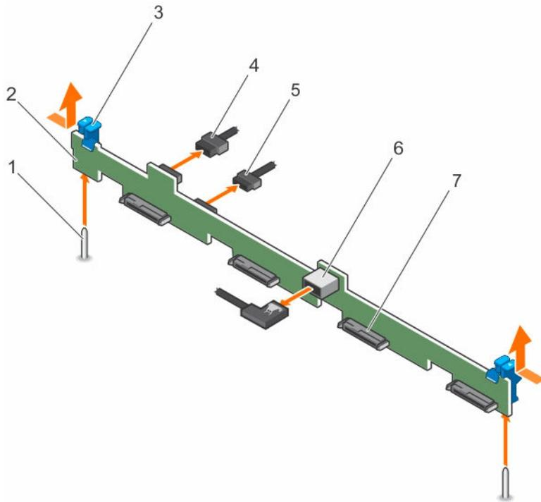
**Figure 78. Removing the four 3.5 inch hard drive SAS/SATA backplane**
