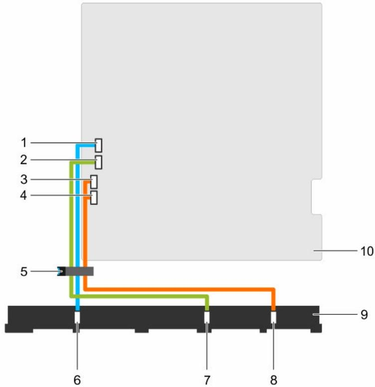
**Figure 83. Cabling diagram—Ten 2.5 inch SAS/SATA backplane**
