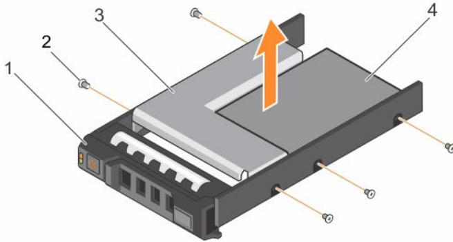
**Figure 36. Removing a 3.5-inch hot swappable hard drive adapter from a 3.5-inch hot swappable hard drive carrier**
