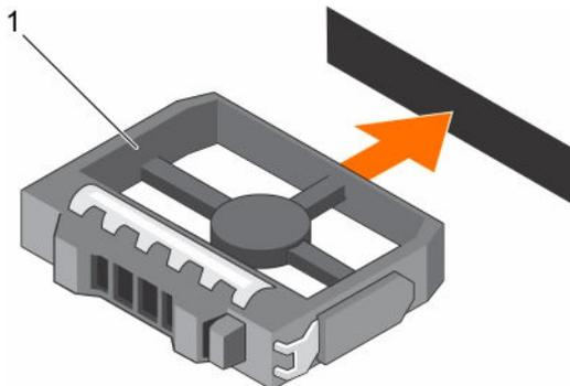
**Figure 31. Installing a 3.5-inch hard drive blank**
