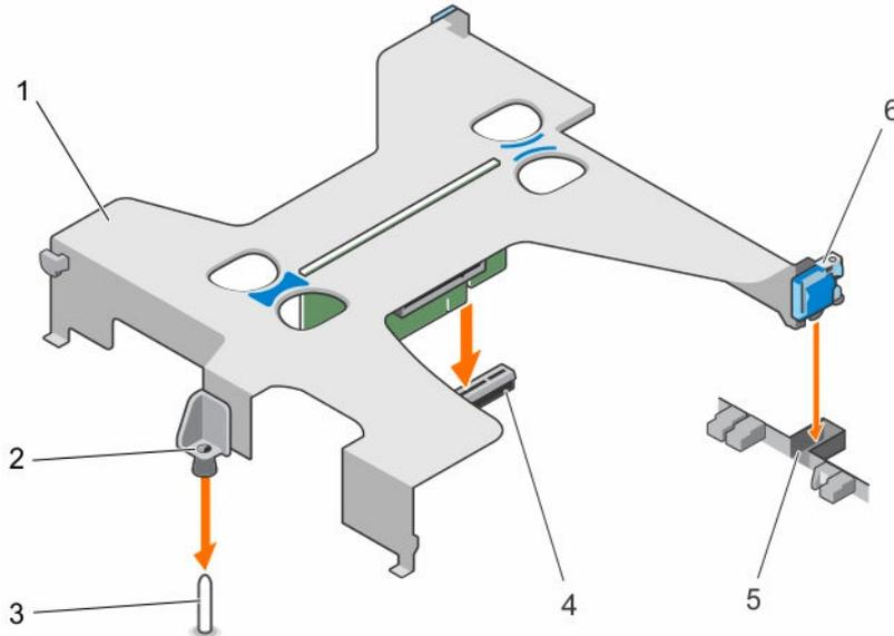
**Figure 51. Installing the expansion card riser**
