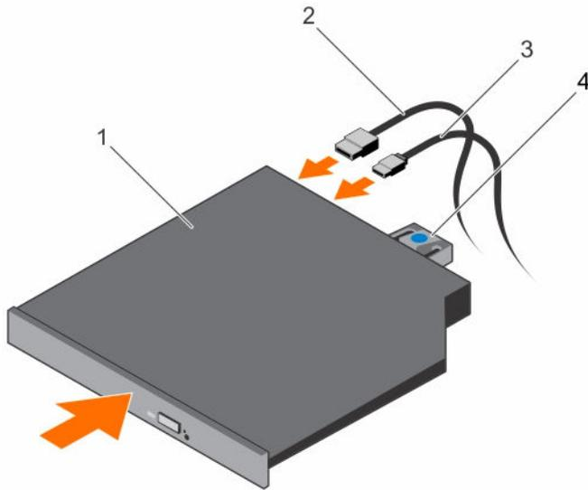
**Figure 43. Installing the ultra slim optical drive**
