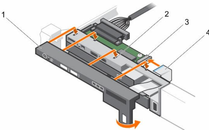
**Figure 91. Installing the control panel—eight 2.5 inch hard-drives/SSDs chassis**
