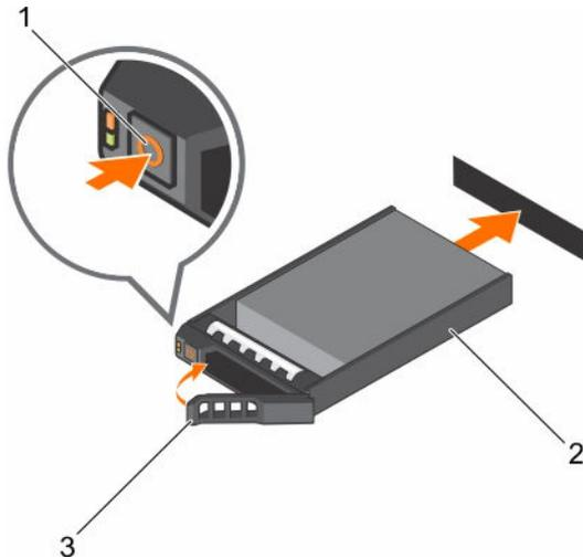
**Figure 35. Installing a hot swappable hard drive carrier**
