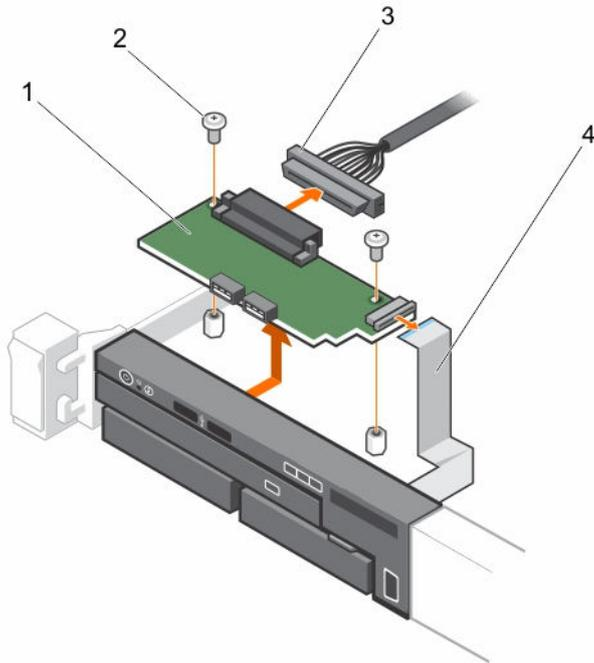
**Figure 95. Removing the control panel module—eight hard-drive chassis**
