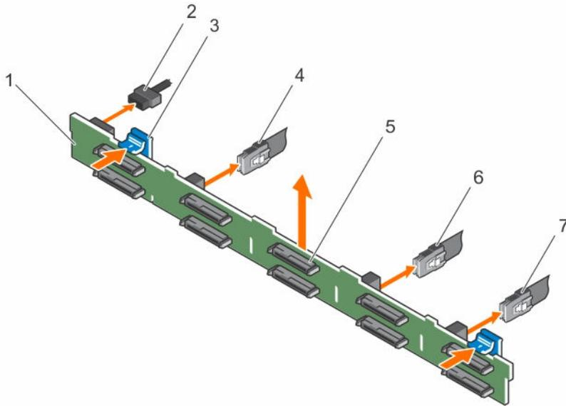
**Figure 82. Removing the ten 2.5 inch SAS/SATA backplane**
