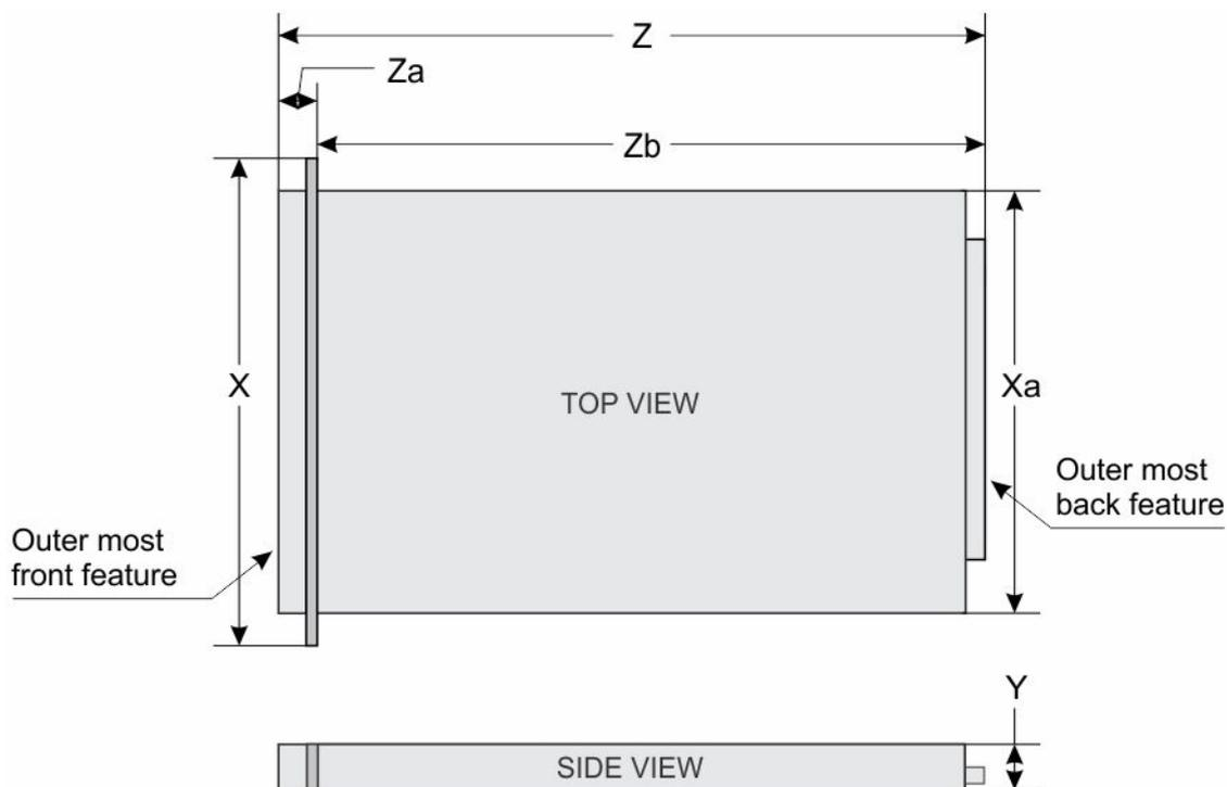
Figure 16. Chassis dimensions of the PowerEdge R430 system
