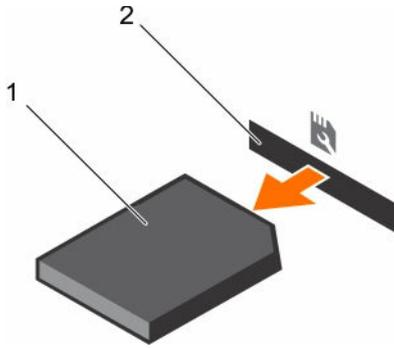
Figure 56. Removing the optional SD vFlash card
