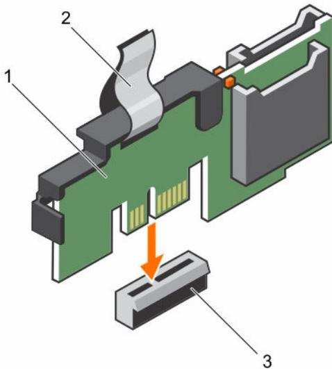
**Figure 61. Installing the optional internal dual SD module**
