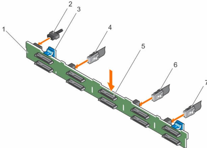
**Figure 86. Installing the ten 2.5 inch SAS/SATA backplane**
