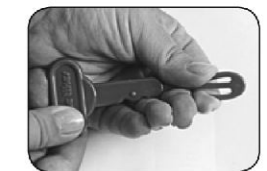
Squeeze the end of key to push through ignition base.
