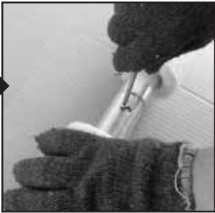
Secure two curved arch tubes together using a self locking screw (M). Tighten with a screwdriver (Q). Then, slide the foam pieces (V) together to cover the screw.
