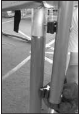
Pull the safety pad (C) over the mat (A), but do not secure it to the top rail (H).
