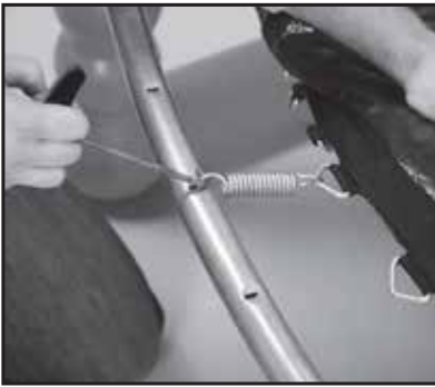
Attach the R-hook galvanized spring (K) with "R" hook end to the triangle-ring on the mat as shown. Holding the spring at 45 degrees in relation to the mat surface will be much easier to install into triangle-ring. Hold the spring loading tool underhand and pull spring hook towards the point on the top rail frame. Drop hook into frame hole until it latches on completely and tap it down if hook is not completely in the hole.
