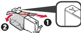
Remove the orange tape completely.
