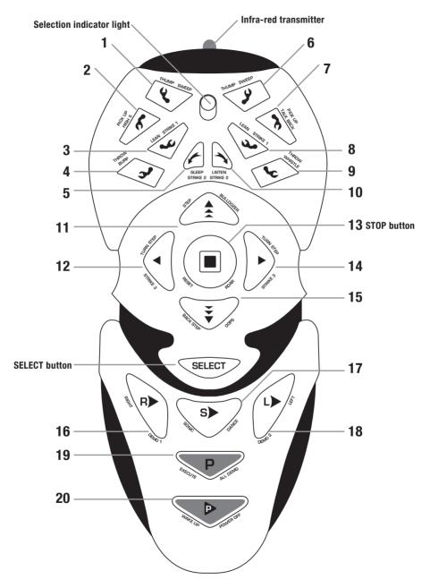
$\label{eq:NOTE: The LEFT side of the Controller operates Robosapien $X^{\text{TM}}$ 's RIGHT side; the RIGHT side of the Controller operates Robosapien $X^{\text{TM}}$ 's LEFT side.}$
