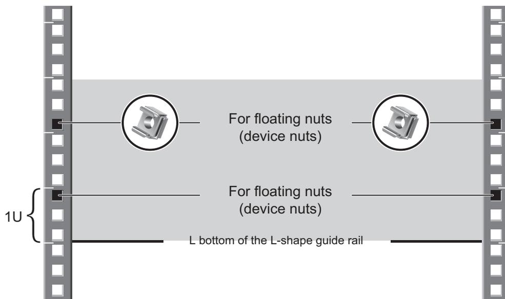
**Figure 3-57** Positions of adjustable guide rails 21241561 and floating nuts
