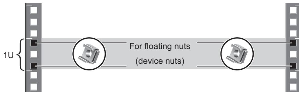
Use M6 screws to fix the floating nuts at the positions specified in **Figure 3-22**, as shown in **Figure 3-23**.
