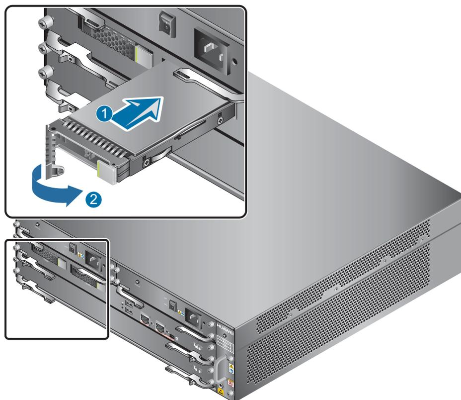
**Step 3** Wait about one minute, and then run the **reset raid primary-disk *disk-id*** command in the system view to create the RAID on the primary disk and synchronize data. In this example, run the **reset raid primary-disk 0** command. Several hours later, run the **display disk information** command. If **Filesystem Status** is **Mounted** and **DiskRaidMode** is **ACTIVE**, both hard disks work properly.
