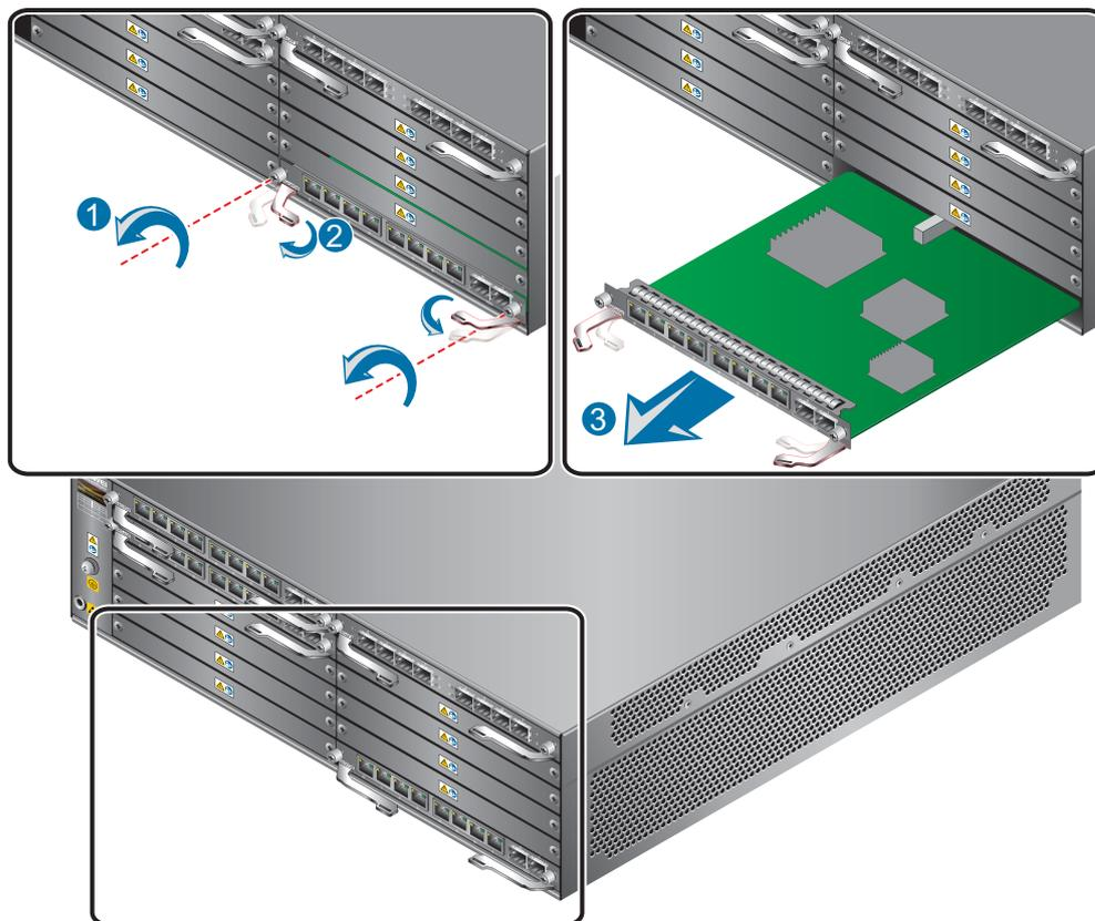
3. Place the removed expansion card into an ESD bag.
