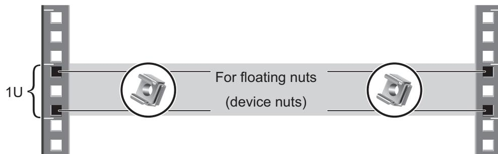
Use M6 screws to fix the floating nuts at the positions specified in [Figure 3-2](#), as shown in [Figure 3-3](#).
