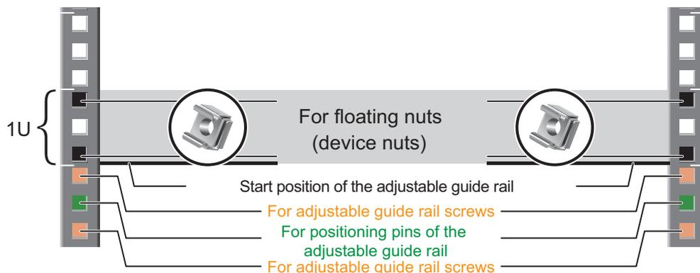
**Figure 3-39** Positions of adjustable guide rails 21242247 and floating nuts
