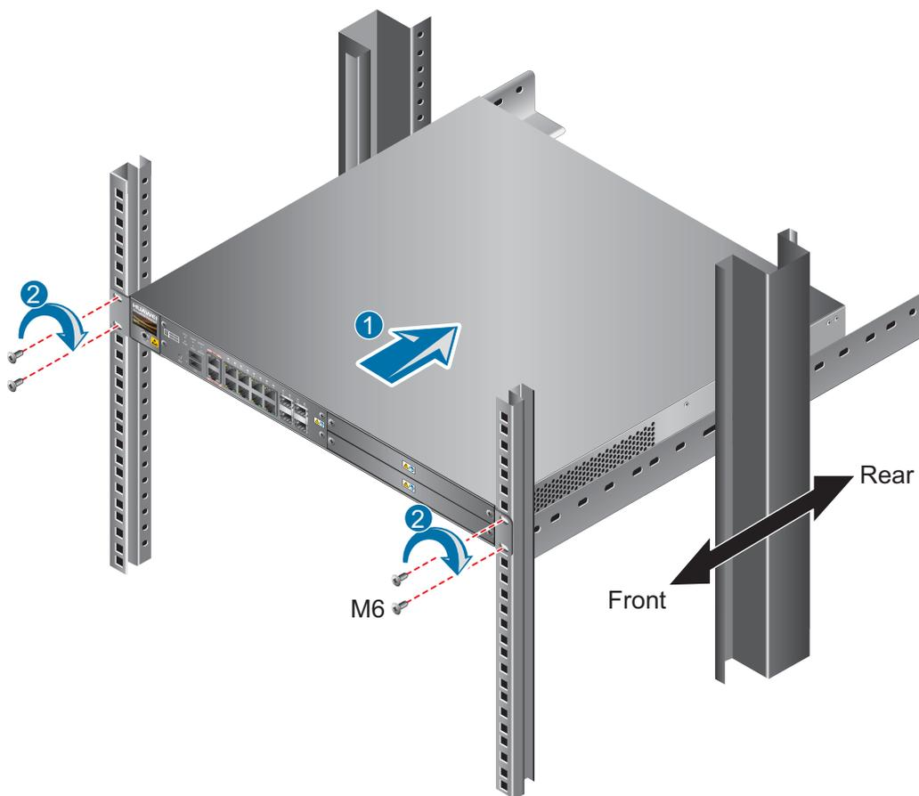
3. (Recommended) For adjustable guide rail 21242247, fix the air baffle to the guide rail with two M6 screws.
