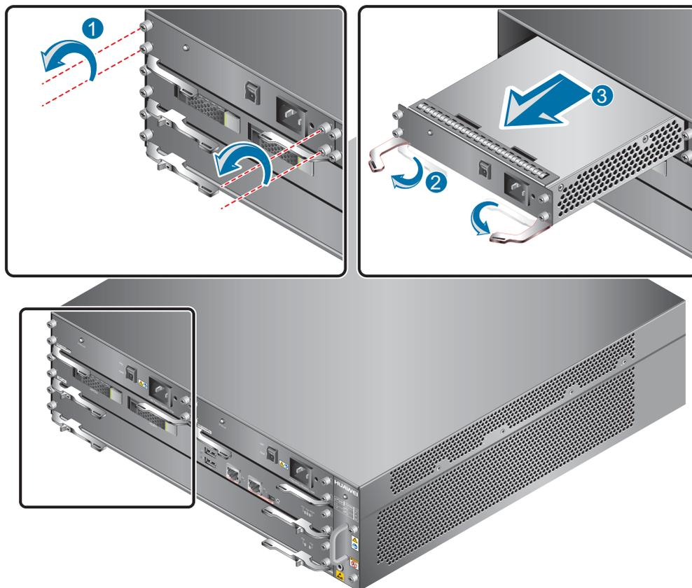
3. Note down the cause and time of the replacement as well as the bar code of the replaced power module and then put away the replaced power module.
