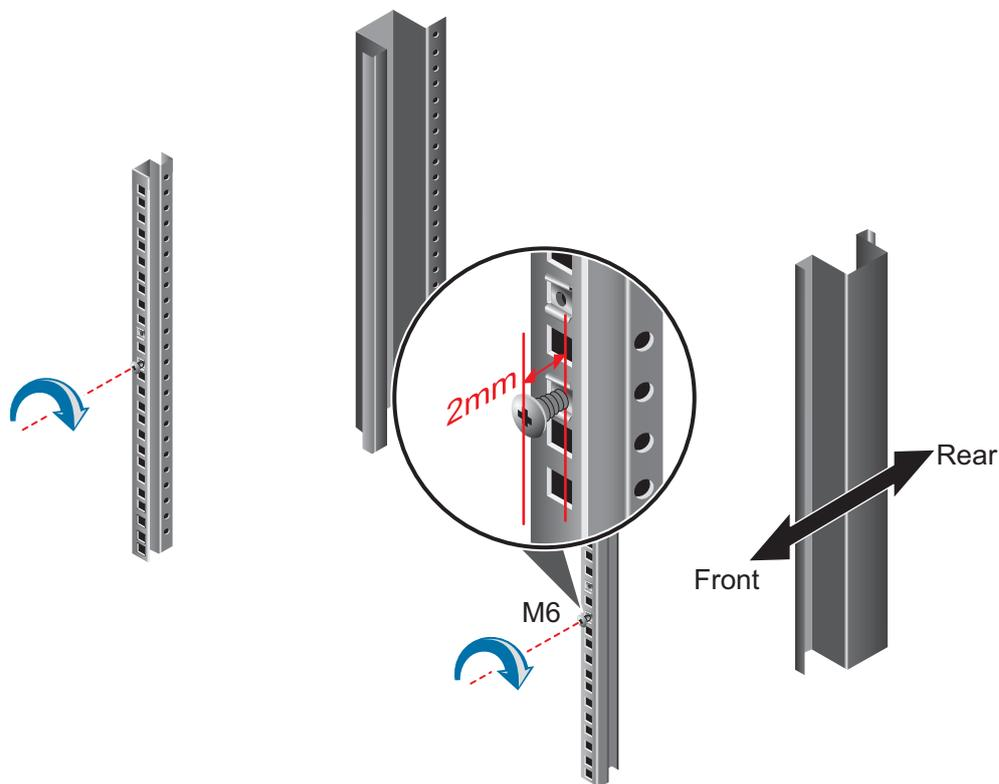
2. Lift the USG, move it to the cabinet, and hang the mounting ears onto the protruding M6 screws.
