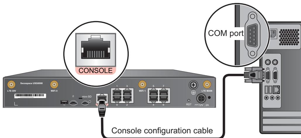
**Step 4** Remove the temporary labels and attach labels 2 cm away from connectors at both ends of the console cable.
