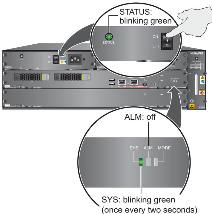
**Figure 3-78** Indicators on the SPUA when the USG6660/6670/6680 (DC model) runs normally
