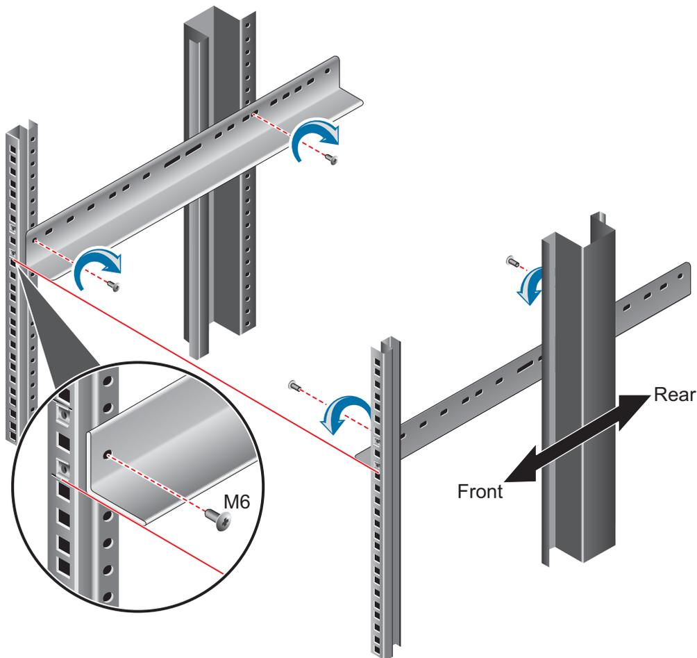
Insert the positioning pins in the front and at the back of the adjustable guide rails 21241561 into the holes at the positions specified in [Figure 3-38](#). Then use the Philips screws to fix the adjustable guide rails inside the cabinet with M6 screws, as shown in [Figure 3-42](#).
