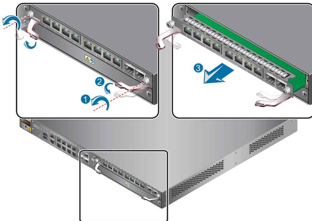
**Figure 4-2** Removing the WSIC expansion card (USG6650/6660/6670/6680)
