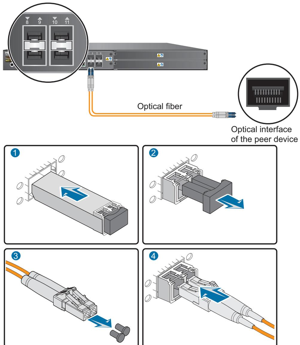
**Step 5** Repeat **Step 1** to **Step 4** to install all optical transceivers and connect all optical fibers.
