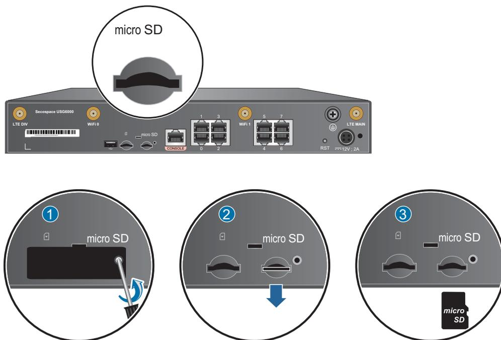
**Step 3** Install the new micro SD card and anti-theft board.
