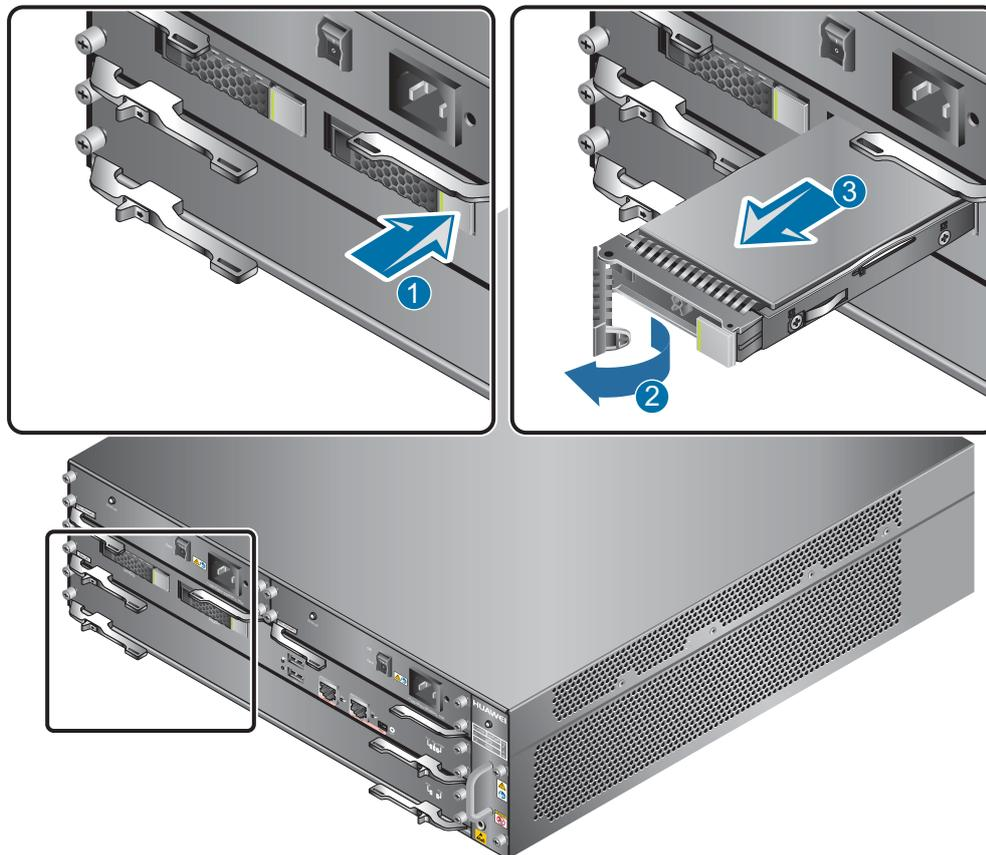
**Step 3** Hold the handlers of the tray and push the tray along the guide rails inside the large-capacity hard disk slot till the tray panel aligns with the panel of the USG. Press the tray handler inwardly to restore the tray.
