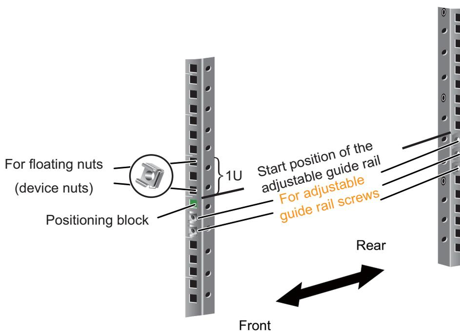
2. Install the floating nuts that match M6 screws at the positions marked in [Figure 3-37](#), [Figure 3-38](#), and [Figure 3-39](#). [Figure 3-40](#) illustrates how to install a floating nut.
