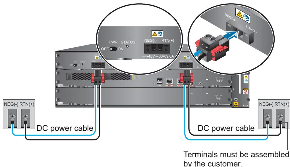
The USG provides cord end terminals and OT bare crimp terminals. You can use them based on the actual condition, including stripping the cable, assembling a terminal, and crimping the cable.
