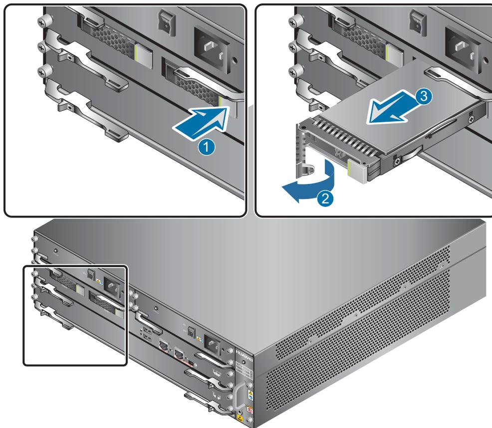
1. Install one large-capacity hard disk in slots HDD0 and HDD1. For example, to install a large-capacity hard disk in slot HDD1, hold the tray handler and push the tray along the guide rails inside the hard disk slot till the tray panel aligns with the panel of the USG. Then press the tray handler inwardly to restore the tray.
