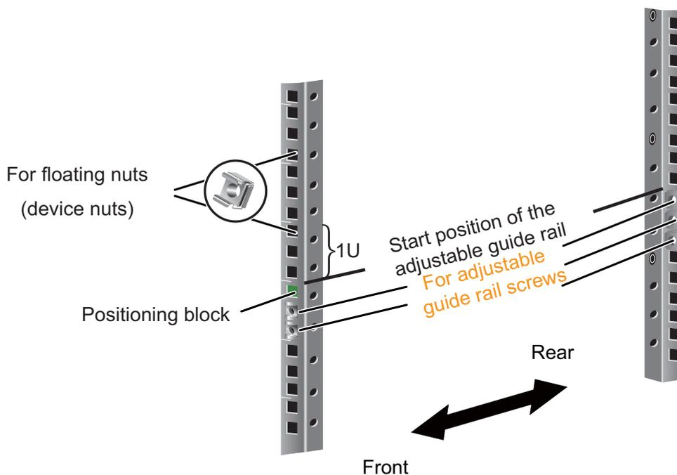
2. Install the floating nuts that match M6 screws at the positions marked in [Figure 3-56](#), [Figure 3-57](#), and [Figure 3-58](#). [Figure 3-59](#) illustrates how to install a floating nut.
