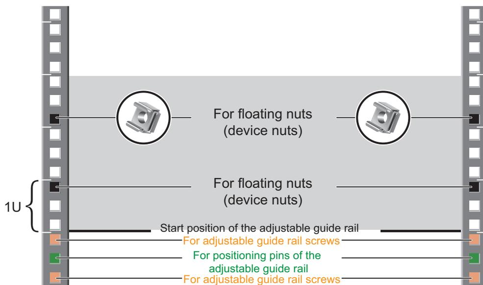
**Figure 3-58** Positions of adjustable guide rails 21242247 and floating nuts
