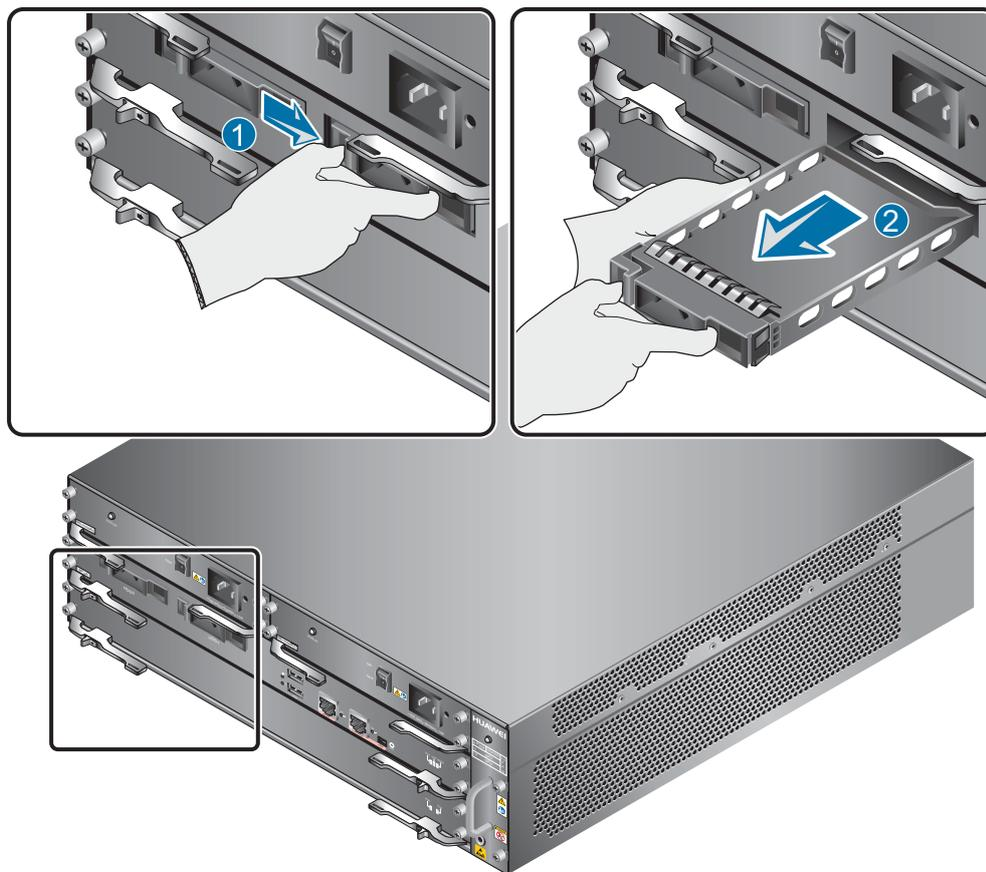
**Step 2** Pull the ejector lever on the hard disk holder and keep it in pulled-out state and push the hard disk holder along the guide rails of the slot till the front surface of the hard disk holder touches the USG panel.
