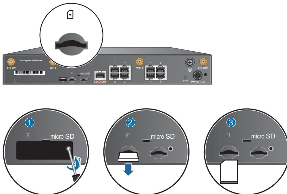
**Step 4** Install the new SIM card and anti-theft board.
