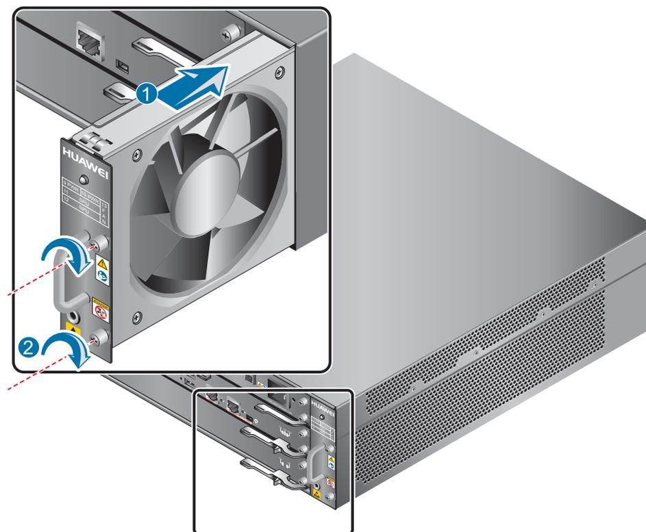
**Step 4** Check the FAN STATUS indicator on the panel. If the indicator is blinking green every two seconds (0.5 Hz), the new fan module works properly.
