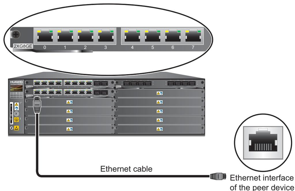
**Step 3** Lay out the Ethernet cable along a cabinet and route the cable through the cable hole for the signal cables at the top (overhead cabling) or bottom (underfloor cabling) of the cabinet.
