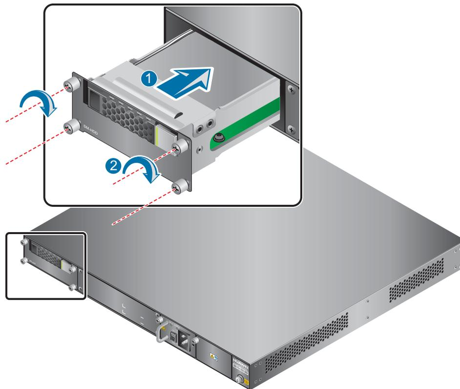
**Step 5** Power on the device, run the **display disk information** command. If **Filesystem Status** is **Mounted** and **DiskCapacity\_Total** is a large capacity, the new hard disk combination works properly.
