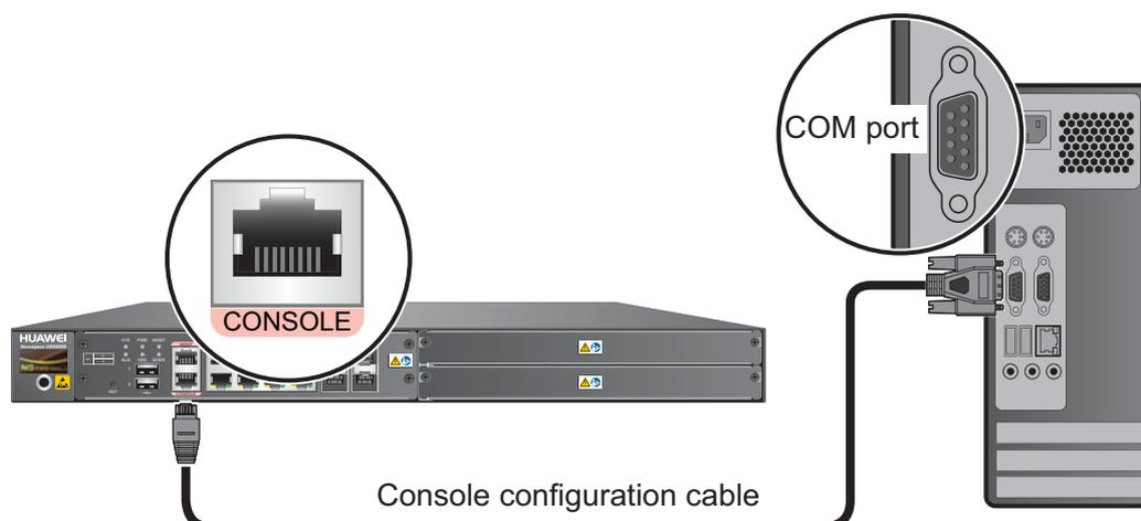
**Step 4** Remove the temporary labels and attach labels (2 cm away from the connectors) at both ends of the console cable.
