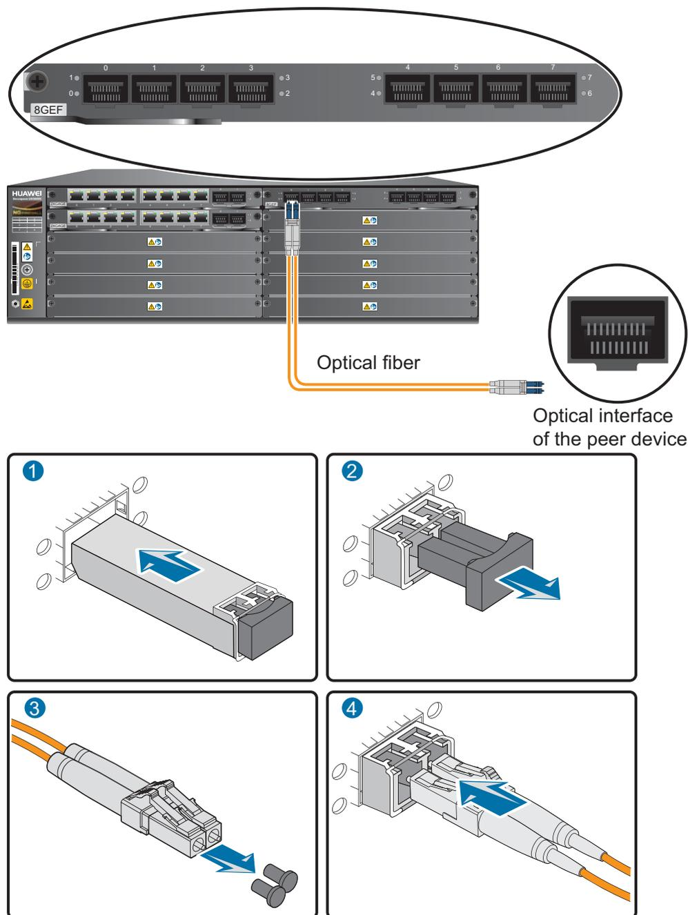
**Step 5** Repeat **Step 1** to **Step 4** to install all optical transceivers and connect all optical fibers.
