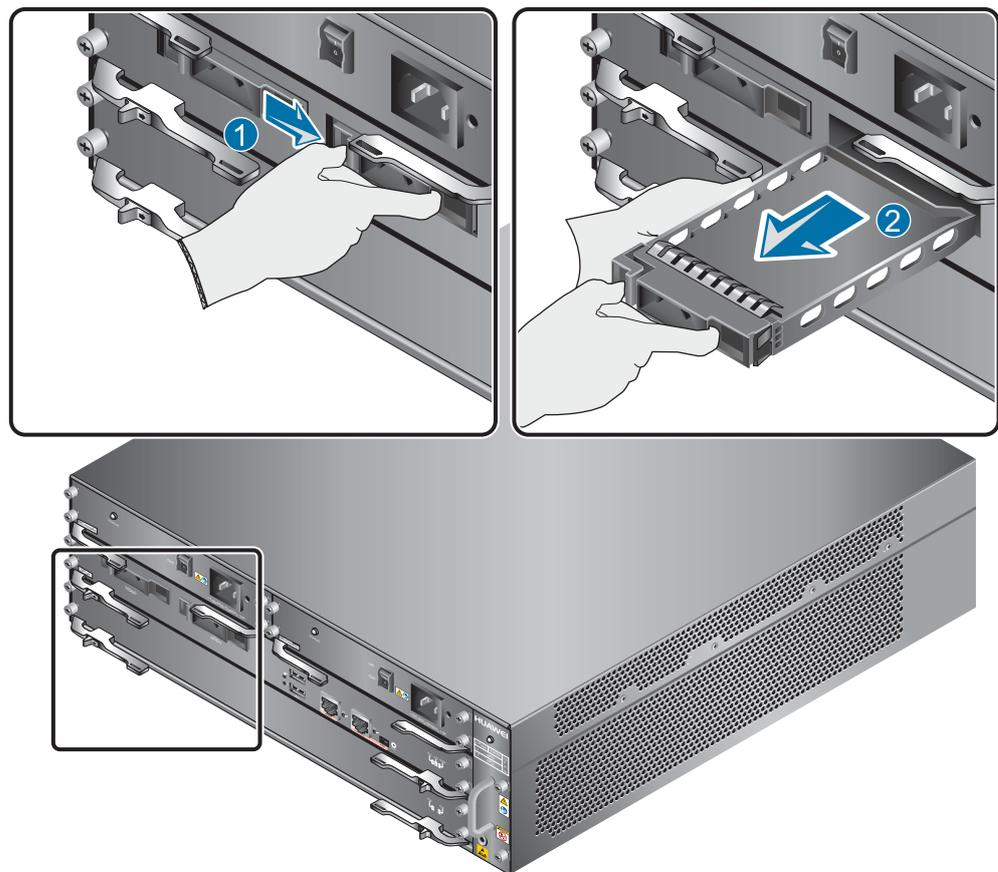
2. Hold the handlers of the tray and push the tray along the guide rails inside the hard disk slot till the tray panel aligns with the panel of the USG.
