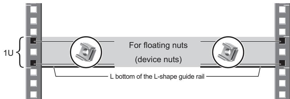
**Figure 3-38** Positions of adjustable guide rails 21241561 and floating nuts
