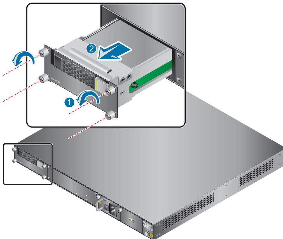
**Figure 4-7** Installing the large-capacity hard disk combination
