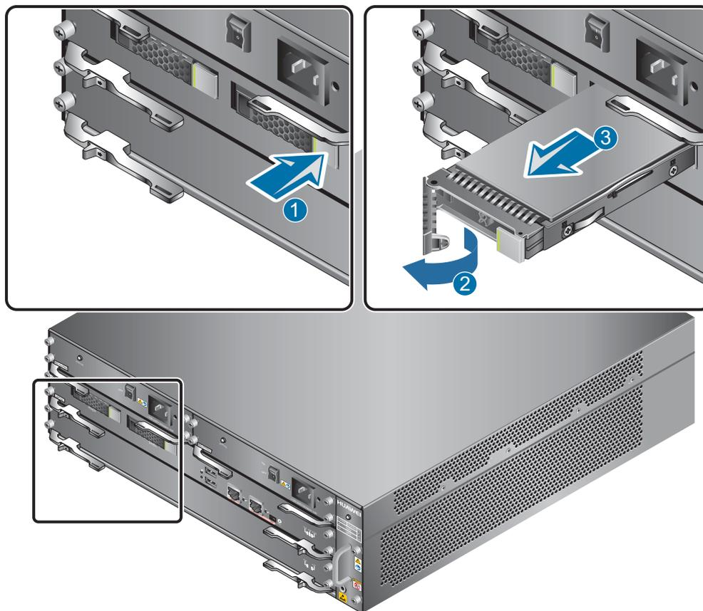
**Step 3** Install one large-capacity hard disk in slots HDD0 and HDD1. For example, to install a large-capacity hard disk in slot HDD1, hold the tray handler and push the tray along the guide rails inside the hard disk slot till the tray panel aligns with the panel of the USG. Then press the tray handler inwardly to restore the tray.
