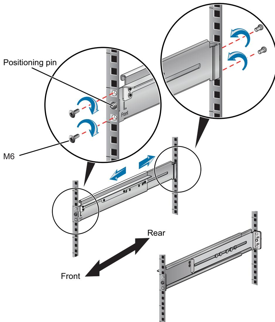
Use the positioning blocks in the front and the positioning hooks at the back of the adjustable guide rails 21242247 as shown in [Figure 3-39](#) to place the guide rails horizontally in the determined installation positions in the racks. Use a Phillips screwdriver to fix the adjustable guide rails to the left and right sides of the cabinet with M6 screws, as shown in [Figure 3-43](#).
