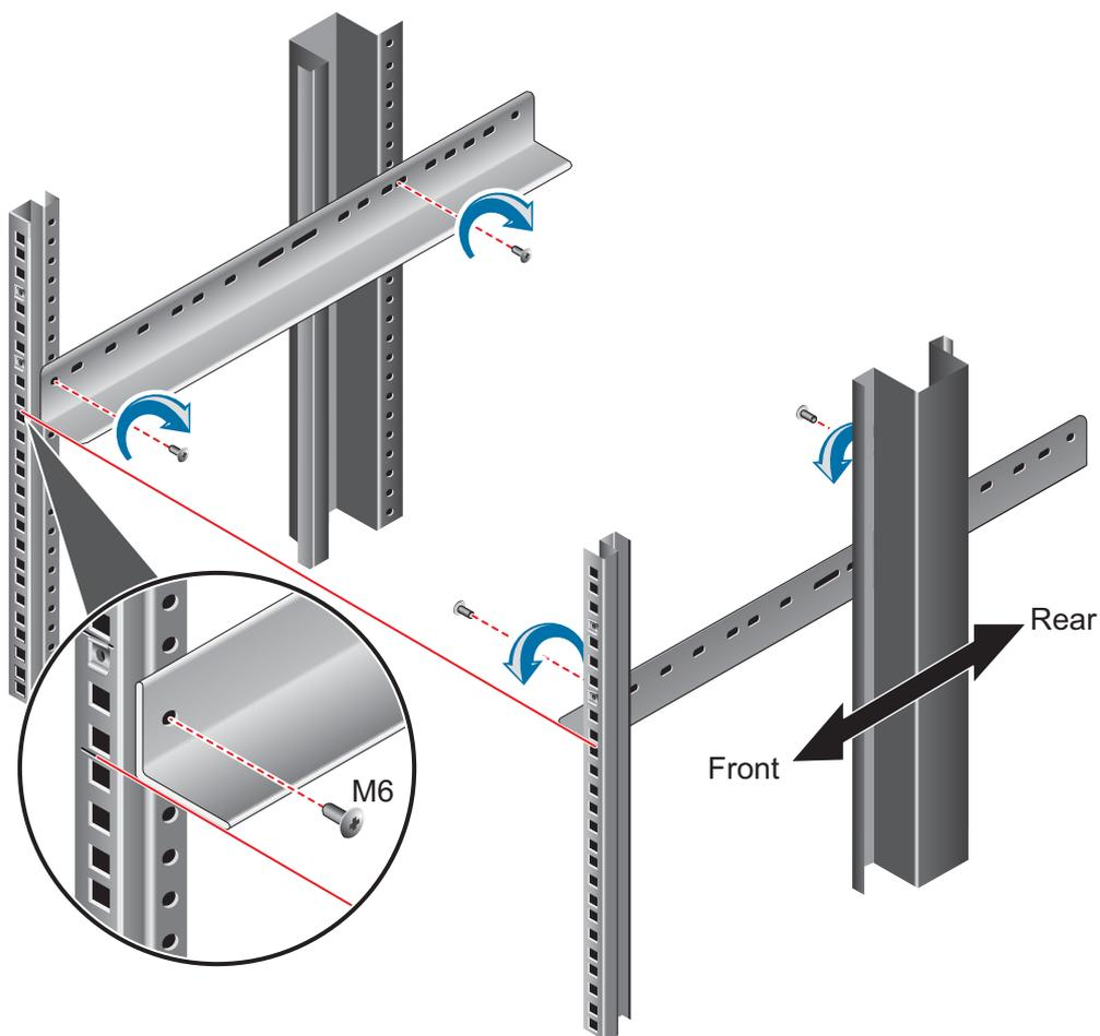
Insert the positioning pins in the front and at the back of the adjustable guide rails 21241561 into the holes at the positions specified in [Figure 3-57](#). Then use the Philips screws to fix the adjustable guide rails inside the cabinet with M6 screws, as shown in [Figure 3-61](#).
