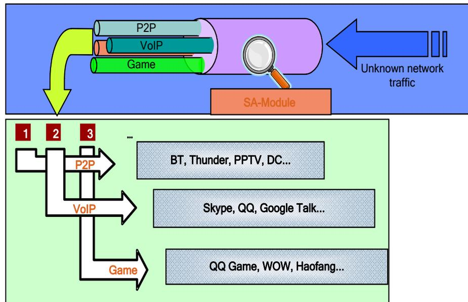
As shown in the previous figure, the application awareness module identifies unknown traffic and packet formats, extracts the signature, payload length, content or length change rule, IP address, and port of a packet, and incorporates statistics on and relationship of packets to accurately categorize applications of the traffic.
