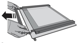
**2.** Lift and firmly hold the inner glass with both hands, remove it and place it on a soft surface before cleaning it.
