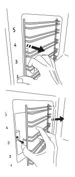
• To reposition the shelf guides, position them near the cavity and initially insert the two pins into their lodgings. Next, position the external part near its lodging, insert the support, and firmly press towards the wall of the cavity to make sure the shelf guide is properly secured.
