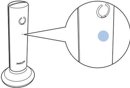
When the handset is placed correctly on the base station, you hear a docking tone when the handset is placed correctly on the base station, you hear a docking tone (see 'Set the docking tone' on page 22). The LED at the back of the handset flashes once.
