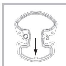
In the case of the Mini WOK burner, use a spanner with a 7 mm opening to unscrew the nozzle (see figure).
