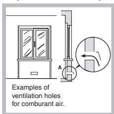
The air circulation system may take air directly from the outside by means of a pipe with an inner cross section of at least  $100 \text{ cm}^2$ ; the opening must not be vulnerable to any type of blockages.
