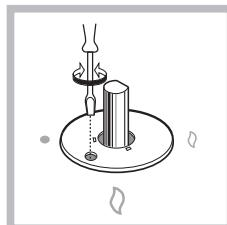
5. Once the adjustment has been made, replace the seals on the by-passes using sealing wax or a similar substance.
