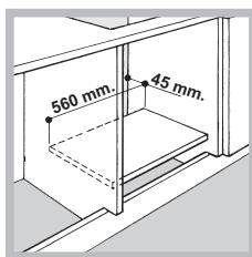
**!** The hob can only be installed above built-in ovens with a cooling ventilation system.
