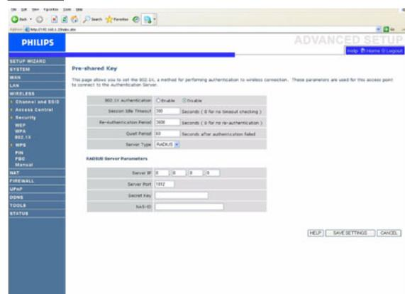
If 802.1x is used in your network, then you should enable this function for the Wireless Router. These parameters are used for the Wireless Router to connect to the authentication server.
