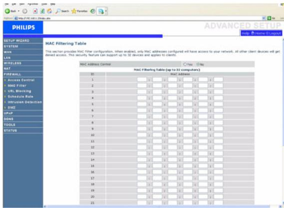
The Wireless Router can also limit the network access based on the MAC address. The MAC Filtering Table allows the Wireless Router to enter up to 32 MAC addresses that are allowed to access to the WAN port.
