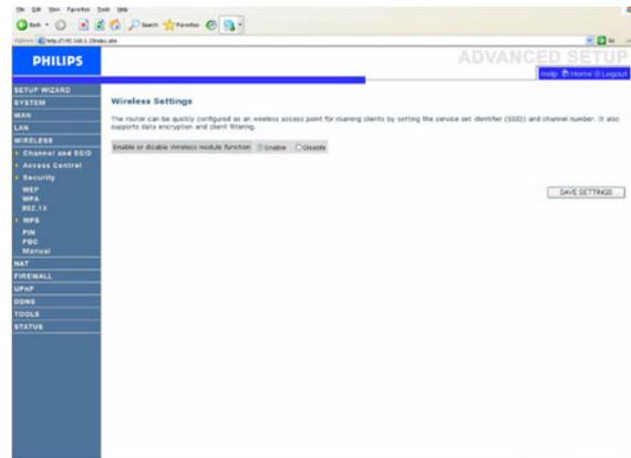
The router can be quickly configured as a wireless access point for roaming clients by setting the service set identifier (SSID) and channel number. It also supports data encryption and client filtering. Check the box to enable the wireless module function.
