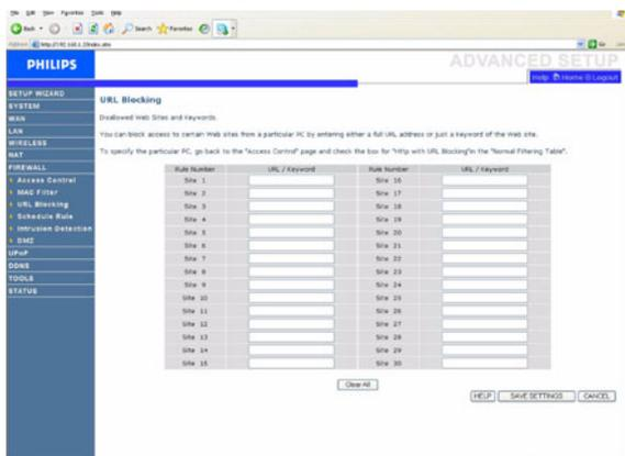
The Wireless Router allows the user to block access to web sites by entering either a full URL address or just a keyword. This feature can be used to protect children from accessing violent or pornographic web sites.
