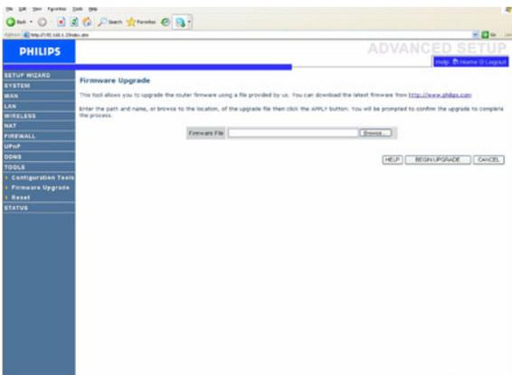
Use the Firmware Upgrade screen to update the firmware or user interface to the latest versions. Download the upgrade file from [www.philips.com/support](http://www.philips.com/support) (Model CAW7740N), and save it to your hard drive. Then click "Browse..." to look for the downloaded file. Click "BEGIN UPGRADE". Check the Status page Information section to confirm that the upgrade process was successful.
