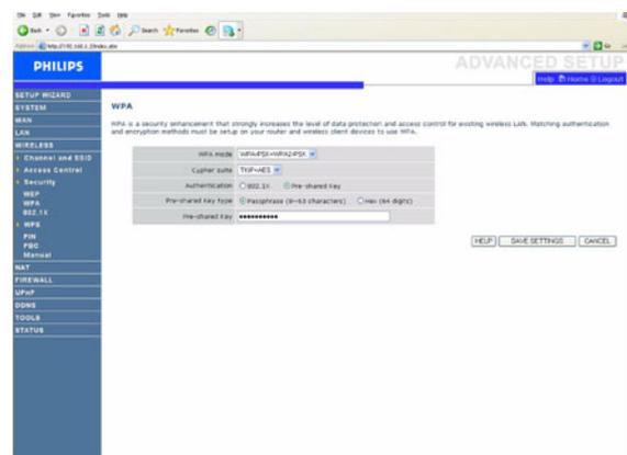
Wi-Fi Protected Access (WPA) combines temporal key integrity protocol (TKIP) and 802.1x mechanisms. It provides dynamic key encryption and 802.1x authentication service.
