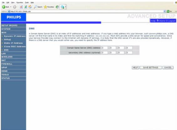
Domain Name Servers (DNS) are used to map a domain name (e.g., www.philips.com) with the IP address (e.g., 64.147.25.20). The DNS address is usually configured automatically. If this is not the case, one or more DNS address will be provided to you by your ISP. However, if there is a DNS server that you would rather use, you need to specify the IP address here.
