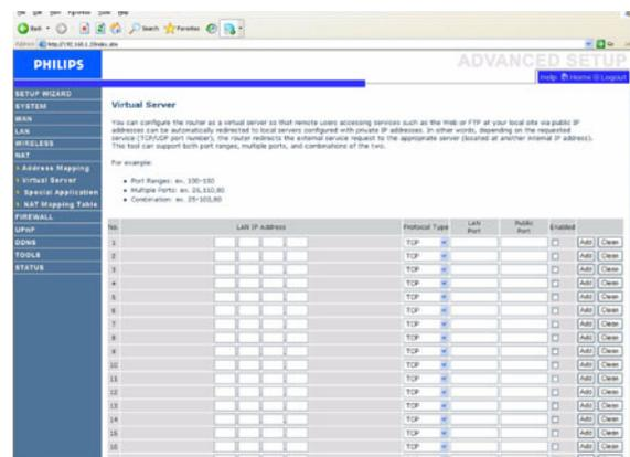
If you configure the Wireless Router as a virtual server, remote users accessing services such as web or FTP at your local site via public IP addresses can be automatically redirected to local servers configured with private IP addresses. In other words, depending on the requested service (TCP/UDP port number), the Wireless Router redirects the external service request to the appropriate server (located at another internal IP address).
