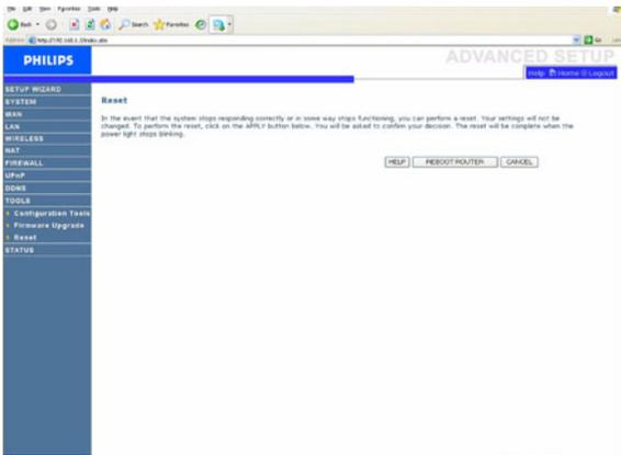
Click "REBOOT ROUTER" to reset the Wireless Router. If you perform a reset from this page, the configuration will not be changed back to the factory default settings.
