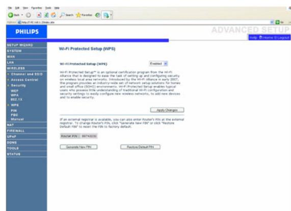
Wi-Fi Protected Setup (WPS) enables typical users who possess little understanding of traditional Wi-Fi configuration and security settings to easily configure new wireless networks, to add new devices and to enable security.
