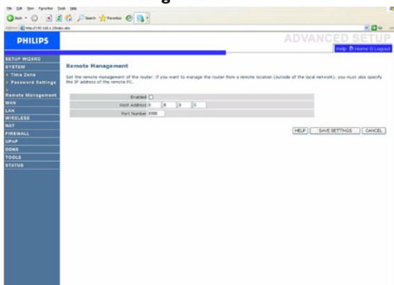
By default, management access is only available to users on your local network. However, you can also manage the Wireless Router from a remote host by entering the IP address of a remote computer on this screen. Check the Enabled check box, and enter the IP address of the Host Address and click "SAVE SETTINGS".
