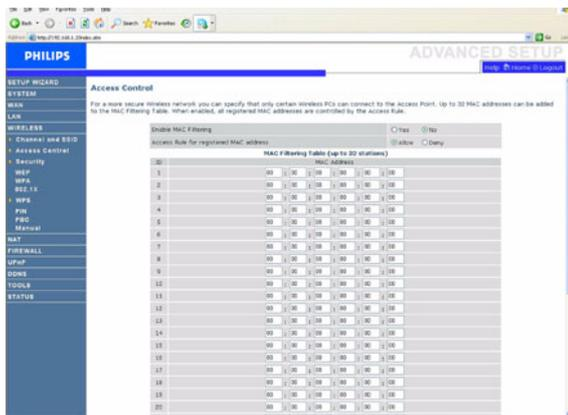
Access Control allows users to define the outgoing traffic permitted or not-permitted through the WAN interface. The default is to permit all outgoing traffic.
