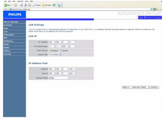
You can enable DHCP to dynamically allocate IP addresses to your client PCs, or configure filtering functions based on specific clients or protocols. The router must have an IP address for the local network.
