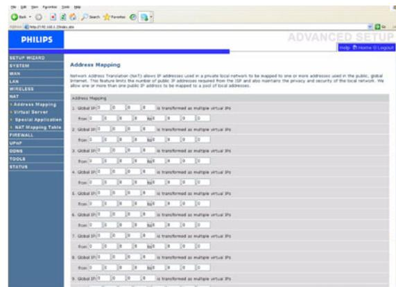
Allows one or more public IP addresses to be shared by multiple internal users. This also hides the internal network for increased privacy and security. Enter the Public IP address you wish to share into the Global IP field. Enter a range of internal IPs that will share the global IP into the "from" field.
