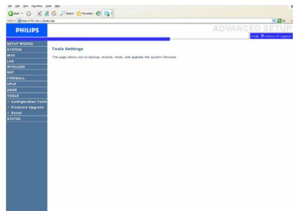
Use the Maintenance menu to backup the current configuration, restore a previously saved configuration, restore factory settings, update firmware, and reset the Wireless Router.
