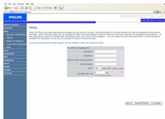
PPPoE is a common connection method used for xDSL.
