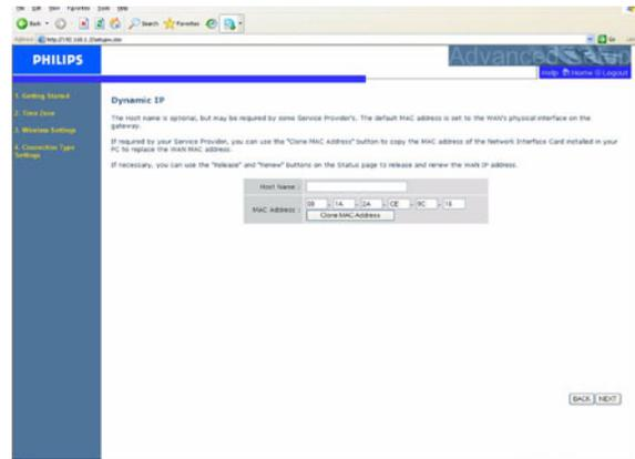
This page allows you to obtain an IP address automatically from your Service Provider.
