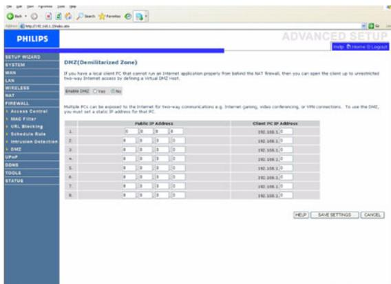
If you have a client PC that cannot run an Internet application properly from behind the firewall, you can open the client up to unrestricted two-way Internet access. Enter the IP address of a DMZ (Demilitarized Zone) host on this screen. Adding a client to the DMZ may expose your local network to a variety of security risks, so only use this option as a last resort.
