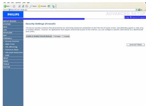
The Wireless Router's firewall inspects packets at the application layer, maintains TCP and UDP session information including time-outs and the number of active sessions, and provides the ability to detect and prevent certain types of network attacks.
