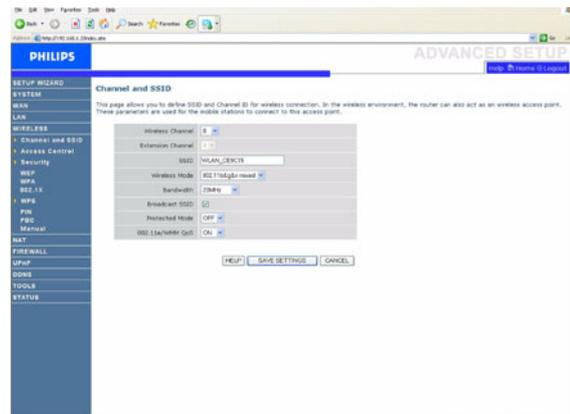
You must specify a common radio channel and SSID (Service Set ID) to be used by the Wireless Router and all of its wireless clients. Make sure you configure all of its clients to the same values.
