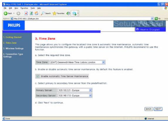
This page allows you to configure the local time zone and automatic time maintenance. Automatic time maintenance synchronizes the router with a public time server on the Internet.
