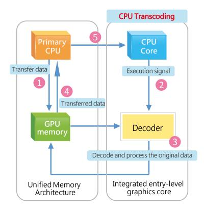
Using video transcoding as an example, a GPU not only reduces the number of data transfers but also processes parallel workloads more efficiently than a CPU.
