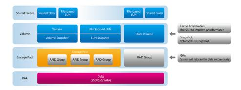
Each layer is designed to cover an aspect of the storage system. The four layers combine to offer you a comprehensive range of options to store and protect your data on your QNAP NAS.
