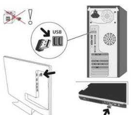
Plug the Mini-USB dongle into the USB port of the TV, PC or notebook. Do not use a hub.
