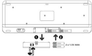
Remove the battery cover and insert 2X 1.5V AAA batteries (included in delivery). Remove the Mini-USB dongle from the allocated space.
