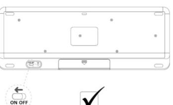
Turn on the wireless keyboard by sliding the slider to "On", which also generates wireless connection. Make sure that the mini USB dongle is plugged into the device and it is switched on.
