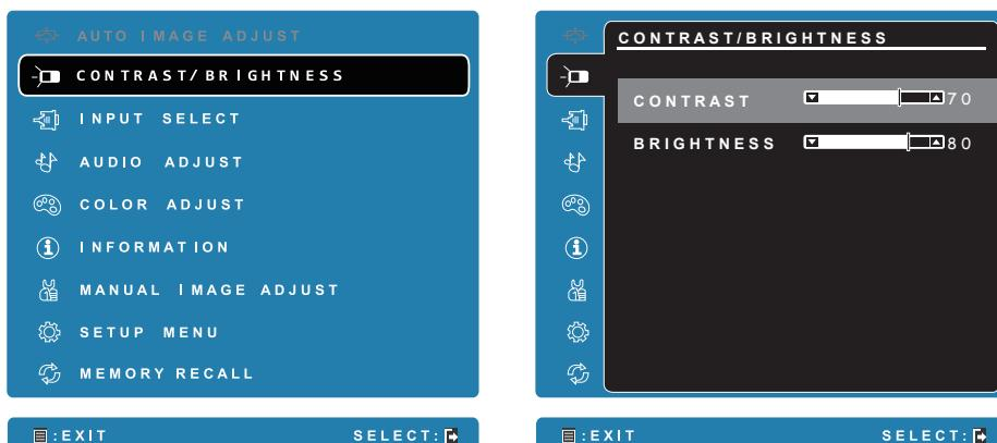
Touch the **Menu/Exit** button on side of your VSD231 to launch OSD configuration screen. The OSD configuration screen can be used to configure the Contrast/Brightness, Input Select, Audio Adjust, Color Adjust, Information, Manual Image Adjust, Setup Menu and Memory Recall.
