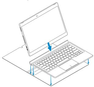
NOTE: The keyboard backlight turns on for 2 seconds when the tablet-docking pins and keyboard-docking pins are aligned correctly.
