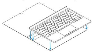
2 Align the tablet-docking pins to the keyboard-docking pins and dock the tablet to the keyboard dock.
