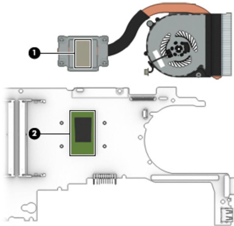
Reverse this procedure to install the heat sink/fan assembly.
