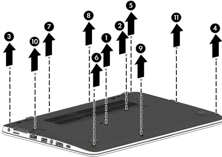
3. Remove the SD card blank and the 1 PM2.0x7.0 screw beneath it **(3)** that secures the bottom cover to the computer.
