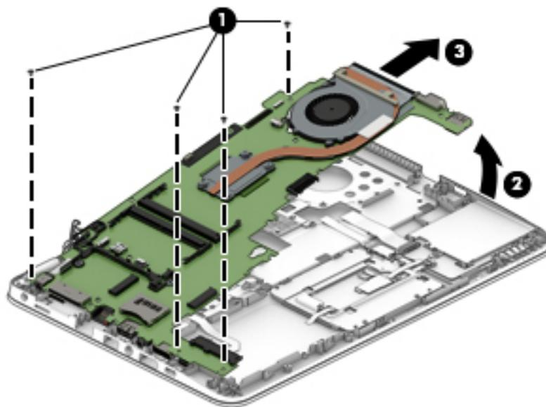
3. Lift the right side of the system board up at an angle **(2)**.
