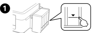
Visually check the ink levels of all ink tanks. If the ink level is below the lower line on the tanks, go to step **2** to refill the tanks.
