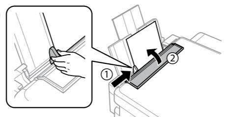
Slide the edge guide against the paper, then close the feeder guard.
