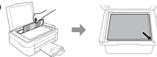
Open the document cover and place your original face-down on the scanner glass. Align the original with the front right corner of the glass.
