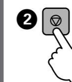
Run print head cleaning until all lines are printed completely. Hold down for 3 seconds until the power light starts flashing. Print head cleaning starts.
