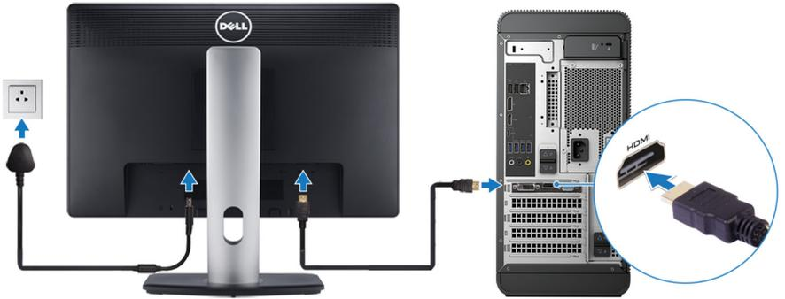
**NOTE:** If you ordered your computer with a discrete graphics card, the HDMI and the display ports on the back panel of your computer are covered. Connect the display to the discrete graphics card.
