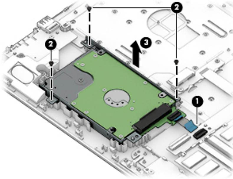
4. To remove the hard drive connector board, pull the connector away from the drive to remove it **(1)**.
