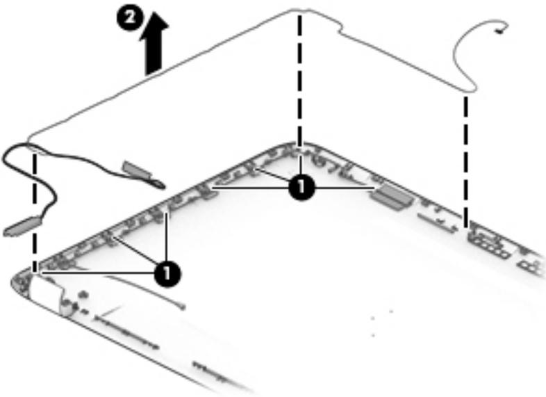
7. If replacing the display enclosure, be sure that the subcomponents (including the webcam/microphone module, the antenna receivers, and all associated cables and hardware) are transferred to the new enclosure.
