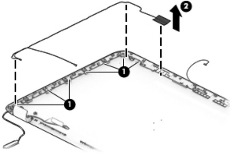
6. To remove the display/webcam cable, remove the cable from the clips built into the display enclosure (1), and then remove the cable from the display enclosure (2).
