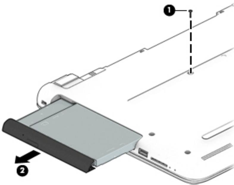
3. If it is necessary to replace the bracket on the rear of the optical drive, remove the two Phillips PM2.0×2.5 screws (1) that secure the bracket to the drive, and then remove the bracket (2).
