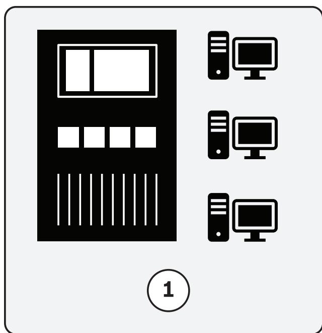
An exclusive Ethernet network in order to set up a central fire alarm network (1) is required. For security and reliability reasons, no networks used for any other purpose (2) may be part of this special network environment. The Fire Monitoring
