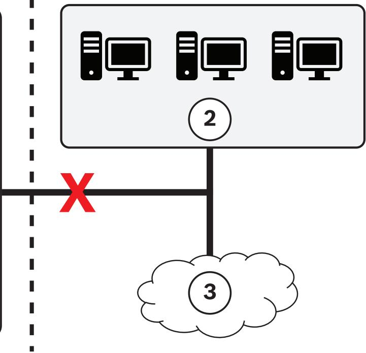
System has to be part of this exclusive fire alarm Ethernet network without direct access to the Internet (3).
