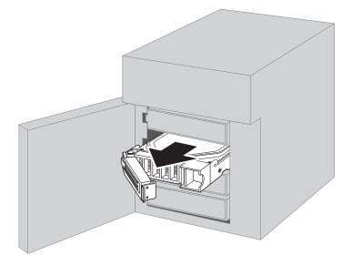
**4** Insert the new drive into the empty slot with the lock mechanism remaining open.
