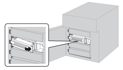
**6** When the replaced drive is recognized, the status LED will flash red and the I31 message will appear on the LCD panel.
