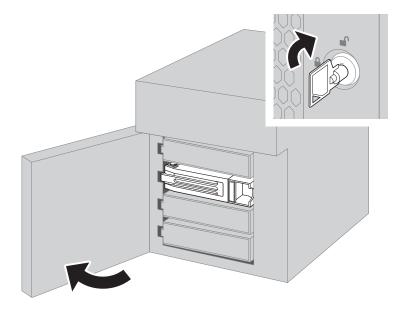
**2** The failed drive's status LED will be glowing red. Push its unlock button and swing the lock mechanism out.
