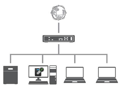
**Note:** For proper operation, make sure that the TeraStation and the authentication server are on a network with only one router. If there are two or more routers on the network, the authentication server may not acquire the correct TeraStation status. For example, if the TeraStation's IP address has been changed, its status does not change to "Warning".
