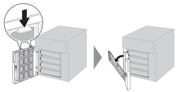
**3** Remove the dustproof filter from the front cover and clear any dust, such as by using a vacuum cleaner.
