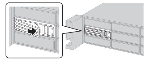
**5** When the replaced drive is recognized, the error LED will flash.
