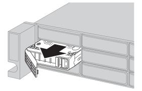
**3** Insert the new drive into the empty slot with the lock mechanism remaining open.
