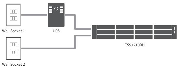
Note: With this connection setup, the option "Wake Up TeraStation After Power Supply Recovers" will not work if it's configured.
