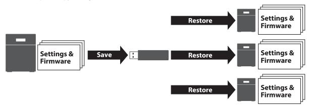
Write down the drive configuration (number of drives, RAID, LVM, etc.) of the TeraStation whose settings were saved. Make sure that any TeraStations that you apply these settings to have the exact same drive configuration before you apply the settings. If the drive configuration is different, you may get unexpected results.
