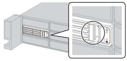
Drives without red error LEDs blinking are still on. Do not unplug or remove them.
