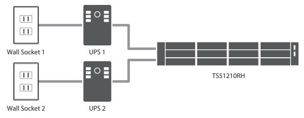
**1** Connect the UPS device and the TeraStation as described above.
