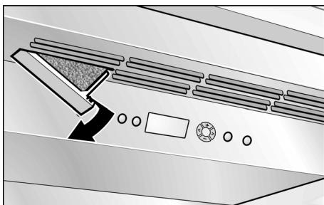
2. Remove the used odour filter and replace with a new odour filter.
