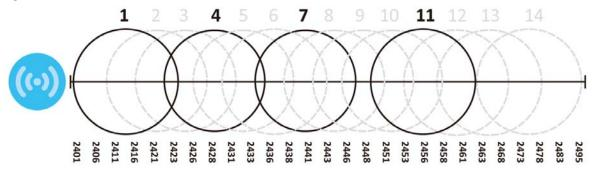
However, some regions require the use of other channels and often use a safety scheme with the following four channels: 1, 4, 7 and 11. While they are situated sufficiently close to both each other and the three so-called "safe" channels (1,6 and 11) that interference becomes inevitable, the severity of it is dependent upon other factors: proximity to the affected AP, signal strength, activity, and so on.
