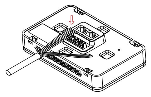
5 Trim any excess wires. Place the dust caps over the terminated wires.
