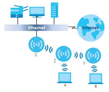
When the NWA/WAC is in Repeater mode, repeater security between the NWA/WAC and other repeater is independent of the security between the wireless clients and the AP or repeater. When repeater security is enabled, both APs and repeaters must use the same pre-shared key. See Section 6.2 on page 70 and Section 10.2 on page 112 for more details.
