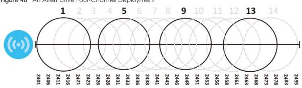
Figure 46 An Alternative Four-Channel Deployment
