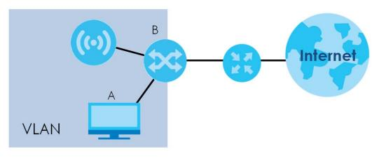
In the figure above, to access and manage the NWA/WAC from computer **A**, the NWA/WAC and switch **B**'s ports to which computer **A** and the NWA/WAC are connected should be in the same VLAN.
