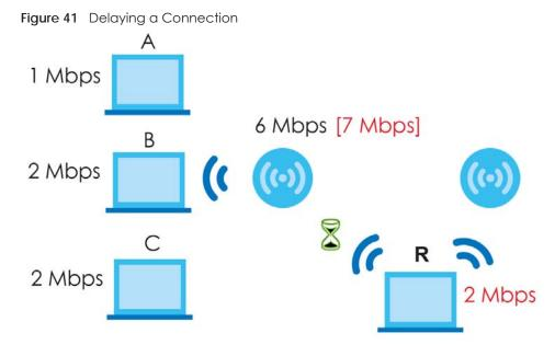
The second response your AP can take is to kick the connections that are pushing it over its balanced bandwidth allotment.
