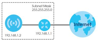
The figure above illustrates one possible setup of your NWA/WAC. The gateway IP address is 192.168.1.1 and the managed IP address of the NWA/WAC is 192.168.1.2 (default), but if the NWA/WAC is assigned an IP address by a DHCP server, the default (192.168.1.2) will not be used. The gateway and the NWA/WAC must belong in the same IP subnet to be able to communicate with each other.
