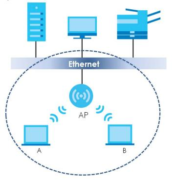
The wireless network is the part in the blue circle. In this wireless network, devices **A** and **B** are called wireless clients. The wireless clients use the access point (AP) to interact with other devices (such as the printer) or with the Internet. Your NWA/WAC is the AP.
