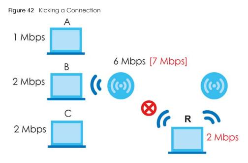
Connections are kicked based on either **idle timeout** or **signal strength**. The NWA/WAC first looks to see which devices have been idle the longest, then starts kicking them in order of highest idle time. If no connections are idle, the next criteria the NWA/WAC analyzes is signal strength. Devices with the weakest signal strength are kicked first.
