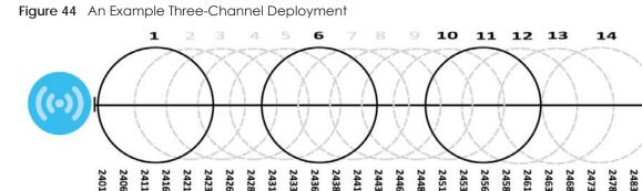
Three channels are situated in such a way as to create almost no interference with one another if used exclusively: 1, 6 and 11. When an AP broadcasts on any of these three channels, it should not interfere with neighboring APs as long as they are also limited to same trio.
