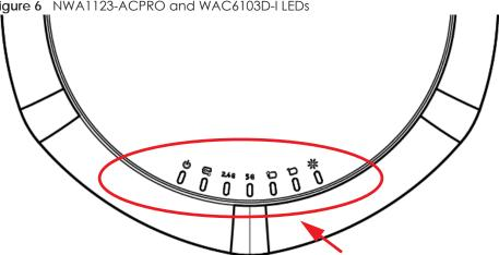
Figure 6 NWA1123-ACPRO and WAC6103D-I LEDs
