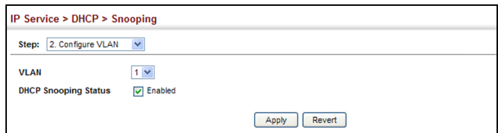
Figure 236: Configuring DHCP Snooping on a VLAN
