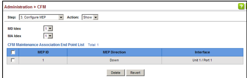
Figure 315: Showing Maintenance End Points
