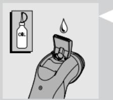
**3** Lubricate the trimmer teeth with a drop of sewing machine oil every six months.
