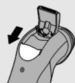
**1** Open the trimmer by pushing the slide downwards.
