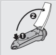
**1** Press the release button (1) and open the cover of the cartridge compartment (2).
