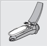
**3** Slide the cartridge with the pump into the shaver. It only fits properly if the white side of the pump is pointing upwards.
