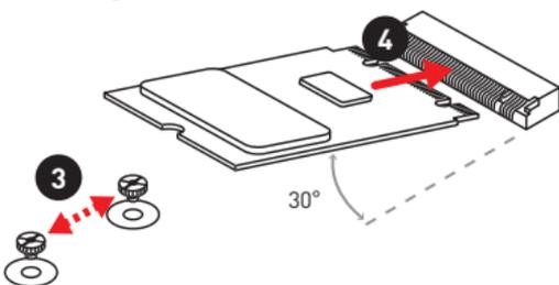
5. Put the screw in the notch on the trailing edge of your M.2 module and tighten it into the base screw.
