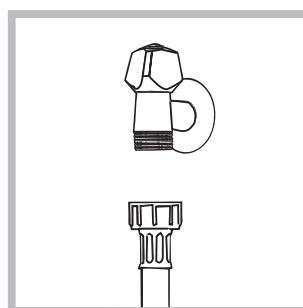
1. Connect the supply pipe by screwing it to a cold water tab using a  $\frac{3}{4}$  gas threaded connection (see figure). Before performing the connection, allow the water to run freely until it is perfectly clear.
