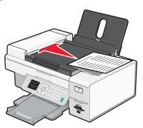
**Note:** Do not load postcards, photos, small items, or thin media (such as magazine clippings) into the Automatic Document Feeder. Place these items on the scanner glass.
