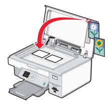
**Note:** For best results, place photos with the most space possible between the photos and the edges of the scan area.
