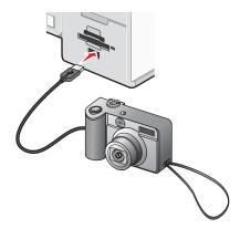
**Warning:** Do not touch the USB cable, any network adapter, or the printer in the area shown while actively printing from a PictBridge-enabled digital camera. A loss of data can occur. Also, do not remove the USB cable or network adapter while actively printing from a PictBridge-enabled digital camera.
