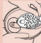
► Put the accessories (emulsifying disc, blade, kneading accessory, insert holder) on the tool holder and store them in the bowl. Always end up with the insert holder.
