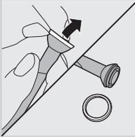
**1** Pull the colour code ring from the bottom of the brush head.
