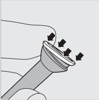
**2** Install a new ring by slipping one edge of the new ring over the bottom of the brush head.
