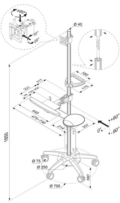
Neomounts Measuring unit: mm
