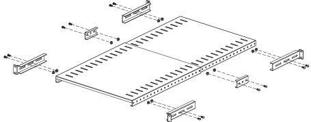
3. Mount the shelf in the rack using the included mounting hardware.
