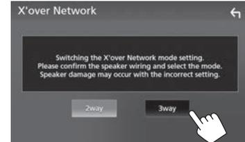
[2 way] Select this when connecting speakers in a 2-way system (front/rear).
