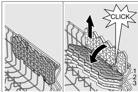
\* Depending on the model, a 3-fold height adjustment is possible. To do this, first place the etagera vertically and pull up, then place at a slight angle, push down to the required height (1, 2, or 3) and snap into place.
