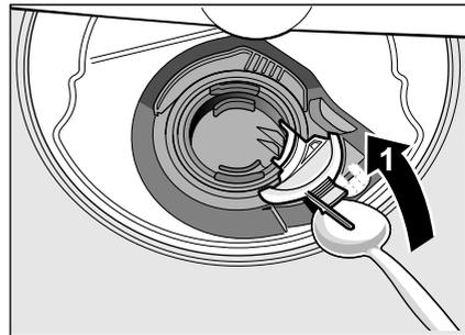
6. Check impeller wheel and remove any foreign objects.
