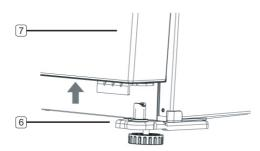
**4.** After the refrigerator is placed to the specified position, install the fridge door in the reverse order as follows:
