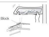
Remove the Vegetable & Fruit Drawer by pressing on the indentations and remove by pulling forward. Holding the drawer with one hand, lift it up a little bit while pulling it forward and take it out of the refrigerator.
