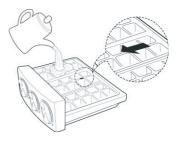
4. Turn twist ice maker button and the ice automatically full into the below ice compartment after release. Pull out ice storage compartment for ice.
