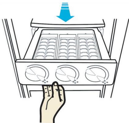
2. Pour cool water into the twist ice maker until it reaches the water level indicator on the ice maker.
