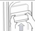
3. Remove the Plastic Drawer by pulling it out and slightly lifting it up.
