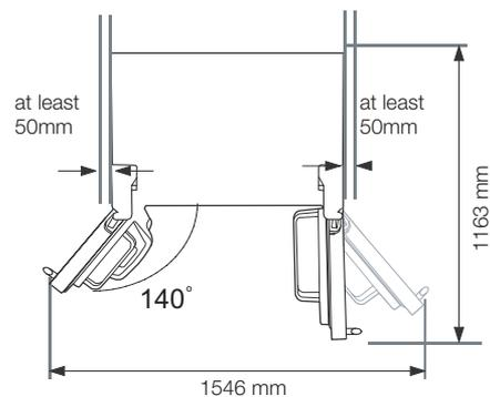
First thing! Make sure that you can easily move your Refrigerator to its final location by measuring doorways (both width and height), thresholds, ceilings, stairways, etc.
