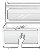
3. Remove the Gallon Door Bin by holding the bin with both hands and gently lifting it up.
