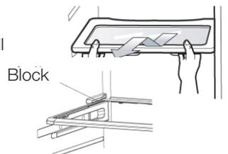
2. Remove the Vegetable & Fruit Drawer by pressing on the indentations and remove by pulling forward. Holding the drawer with one hand, lift it up a little bit while pulling it forward and take it out of the refrigerator.
