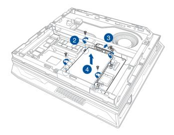
5. Remove the four screws from the bracket and remove it from the HDD/SSD.
