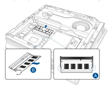
**NOTE:** Use the same model and speed when replacing memory modules.
