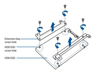
6. Prepare your new HDD/SSD and secure the bracket to it using the four screws removed previously. Ensure that screw holes on the 2.5-inch HDD/SSD matches the screw holes on the bracket.
