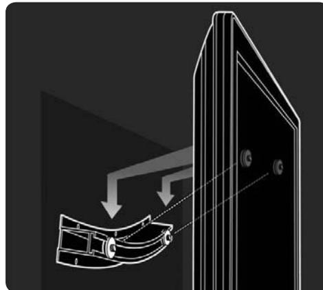
3 Mount the 2 spacers on the 2 lower discs at the back of the TV.
