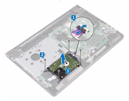
Disconnect the interposer from the hard-drive assembly.
