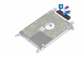
Remove the four screws (M3x3) that secure the hard-drive bracket to the hard drive.
