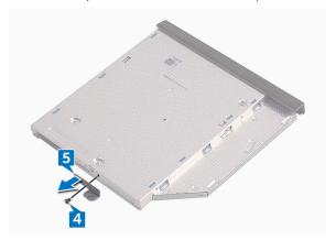
Carefully pull the optical-drive bezel and remove it from the optical drive.
