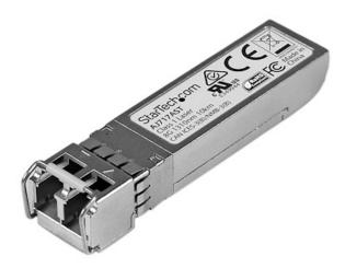
The AJ717AST is an HPE AJ716B compatible fiber transceiver module that has been designed, programmed and tested to work with HPE brand switches and routers. It delivers dependable 8Gb fiber channel connectivity over fiber cable, for 8GFC compliant networks, with a maximum distance of up to 10 km (6.2 mi).
